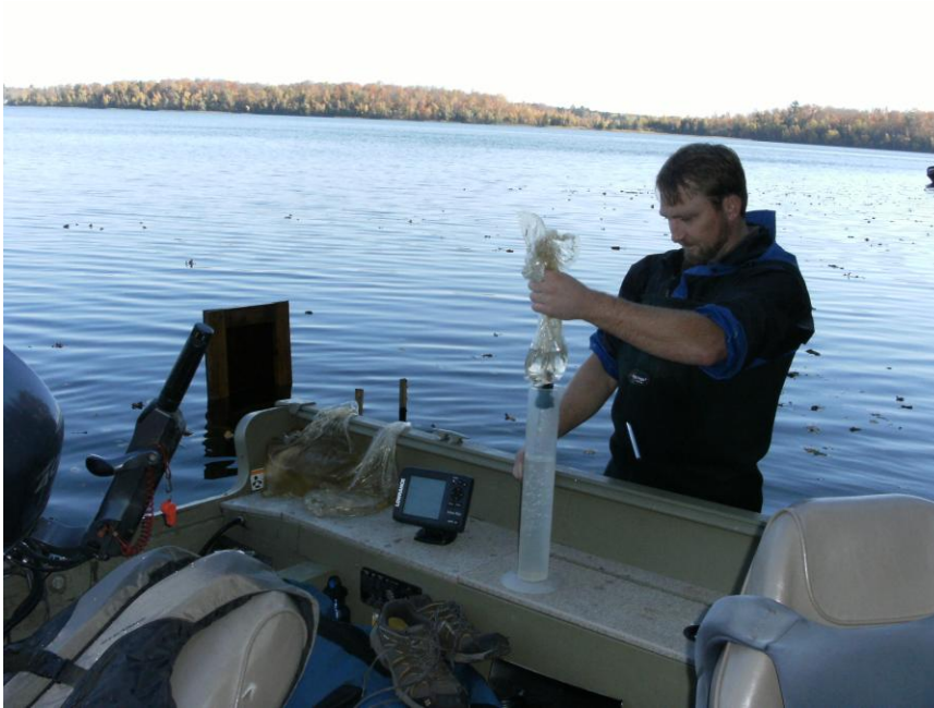
Figure 69: Andy Arens (ISWCD) measures shallow groundwater inflows to Pokegama Lake.
