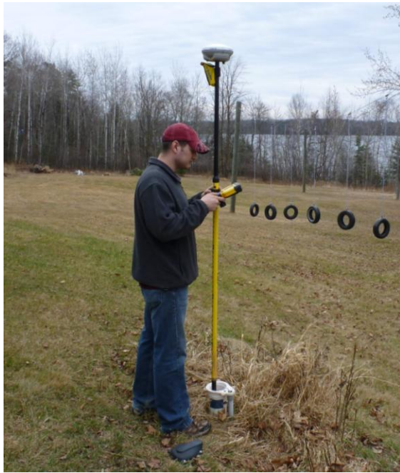
Figure 24: Joey LeBlanc (NRCS) surveying well elevation.
